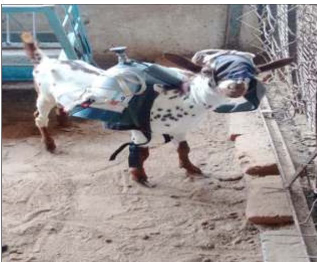
Fig 2 Goat fitted with SF 6 assembly for methane gas estimation
